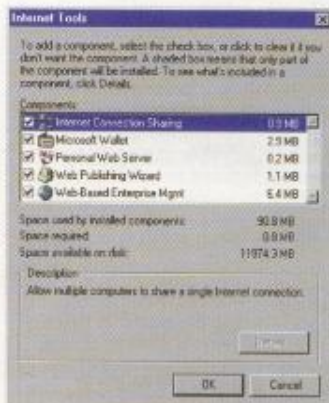
Figure A. - Select the Internet Connection Sharing check box in the Internet Tools dialog box.
