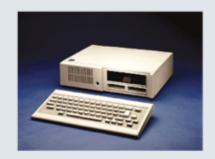
optical link keyboard. The PCjr relied on a television for video output. Running PC-DOS 2.1, the PCjr came with the BASIC programming language, as well as a host of home management, educational, and entertainment software. (An enhanced model released at the same time as the base model came with all these features, yet added another 64KB of RAM; a 5.25-inch, 360KB floppy diskette drive; and a color graphics card that allowed for the use of a color monitor.)
